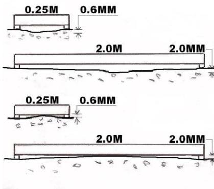
The surface must be smooth; cavities and other roughnesses must be within  $\pm 0.6\text{mm}$  on a 0.25 metre straight-edge.
