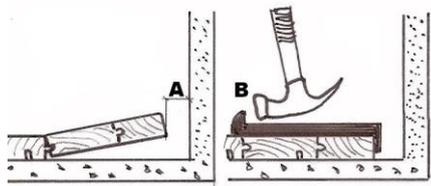
If necessary, use a joint puller (B) to slot the last board into place.
